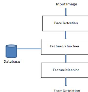
**Figure.1. process of face detection and reorganization**
