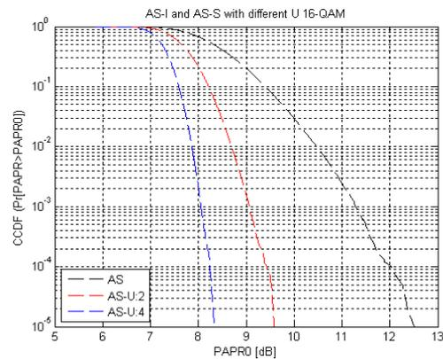
Figure.4. AS-1 and AS-S with different U 16-QAM
