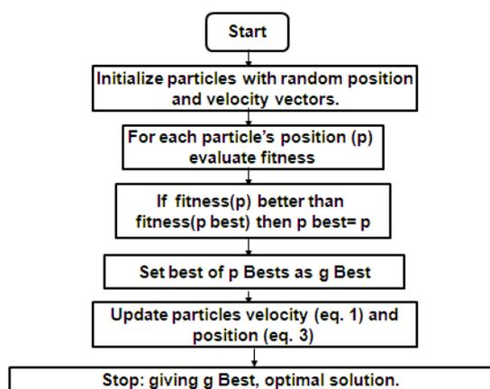
**Figure.2. Flow Chart on PSO Algorithm in MIMO-OFDM System**
