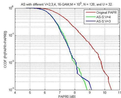
Figure.5. PAPR reduction on AS with different  $V=2;3;4$ , 16-QAM,  $M = 10^3$ ,  $N = 128$ , and  $U = 32$  with SFBC the use of 256QAM
