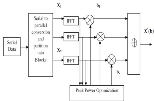
**Figure.1. Block Diagram of Partial Transmit Sequence Technique**
