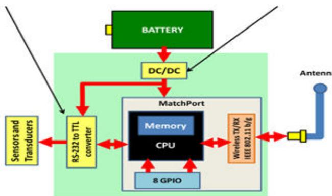
Figure.1 Block diagram of the underwater wireless sensor node.
