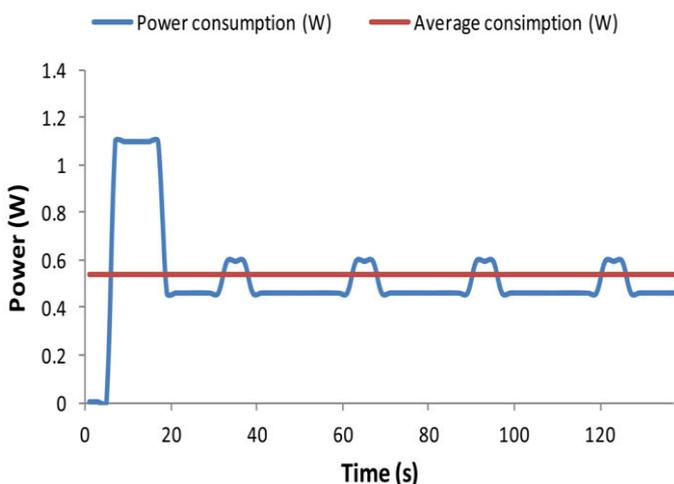
Figure.6. Underwater wireless sensor node consumption.
