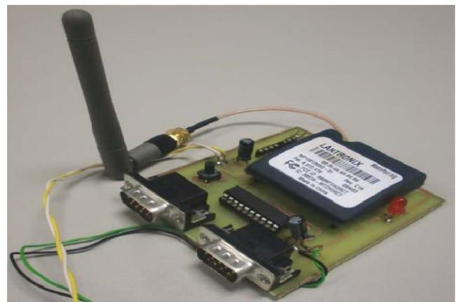
Figure.2 Image of the underwater wireless sensor node.
