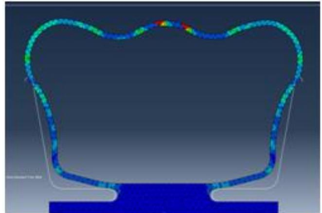
Figure.4. 2<sup>nd</sup> Stage of Seal Inflation
