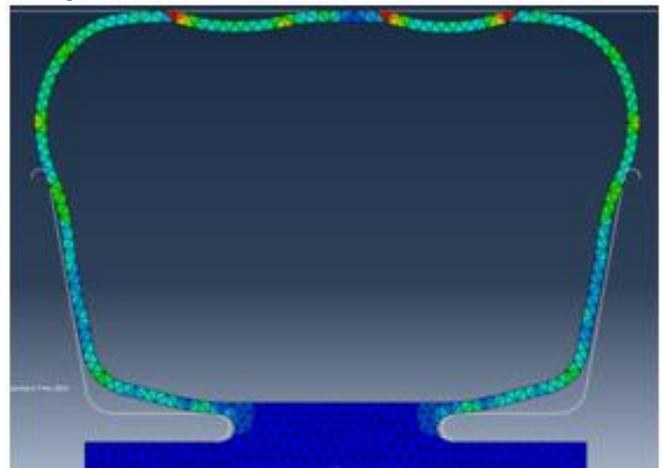
Figure.5. Fully Inflated Seal
