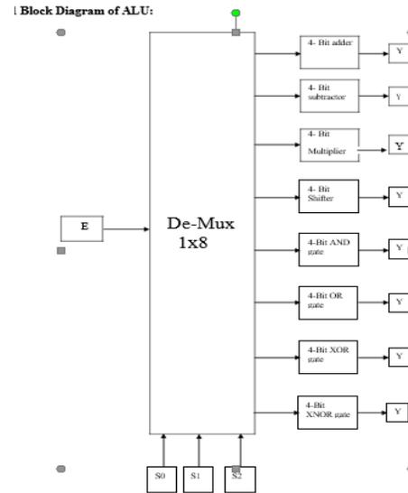
Figure.7. block diagram of ALU
