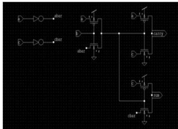
Figure.10. Schematic view of 6T adder
