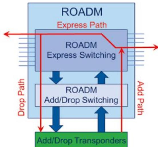
**Figure.1. Express and add/ drop functions of a ROADM**
