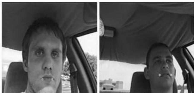
Figure.1. Lip tracking using NIR camera.
