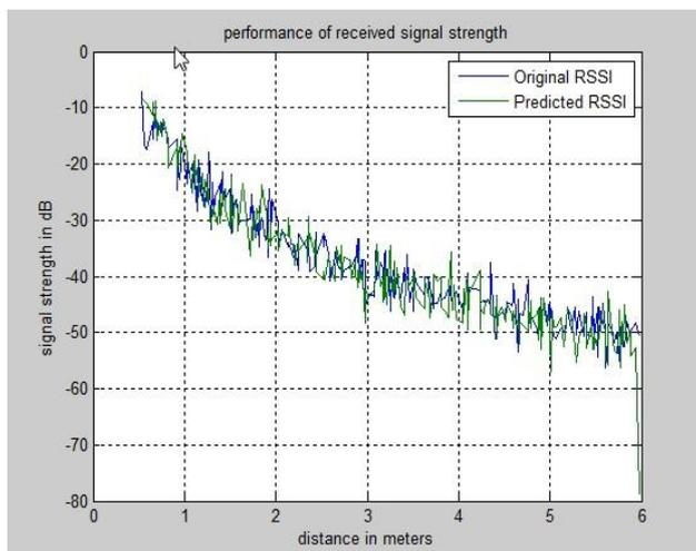
Figure.2. Performance of received signal strength (predicted RSSI)
