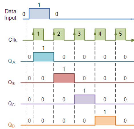
Figure. 3. Existing synchronizer using Serial-In-Parallel-Out and Parallel-in-Serial-out
