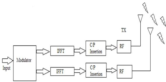
Figure .1.1Block Diagram of OFDM Transmitter
