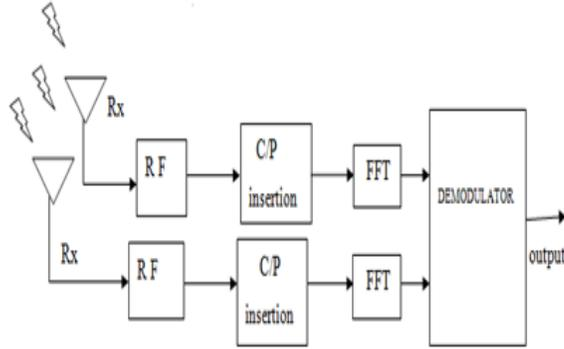
Figure .1.2Block Diagram of OFDM Receiver
