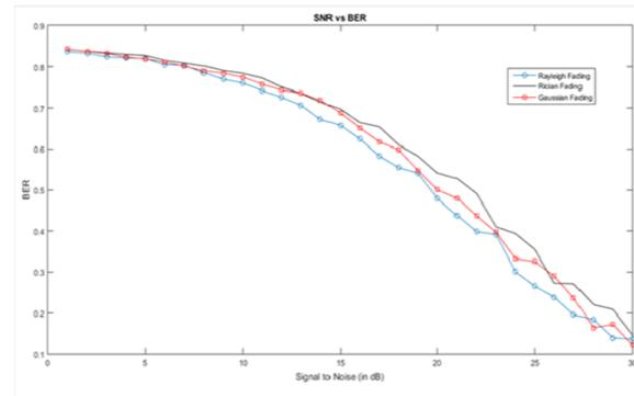
Figure.1.5. Graphical comparison of BER for QAM for different fading channels
