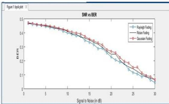
Figure.1.3: Graphical comparison of BER for BPSK for different fading channels
