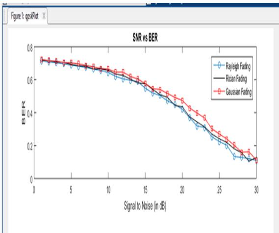
Figure.1.4. Graphical comparison of BER for QPSK for different fading channels
