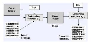
Figure.1. the basic Steganography Model
