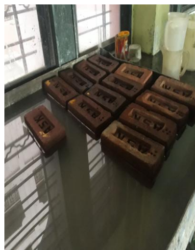
Figure.4. efflorescence test at the laboratory
