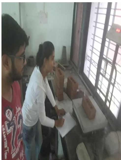
Figure.3. Laboratory testing for water absorption
