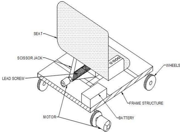
Figure.No 3.1:working diagram
