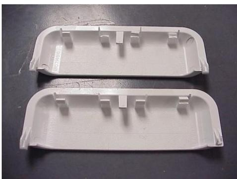
**Figure.20. Broken handle after experimentation**
