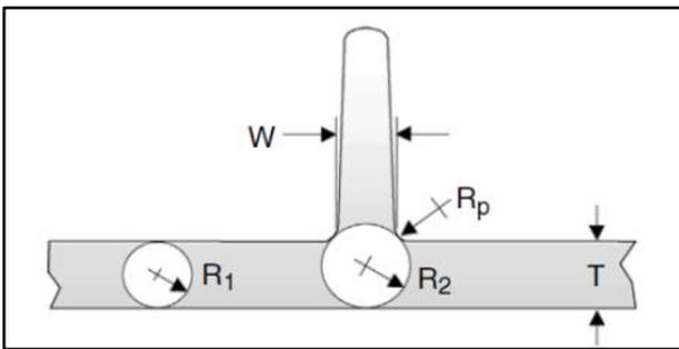
Figure.12. Protrusion thickness
