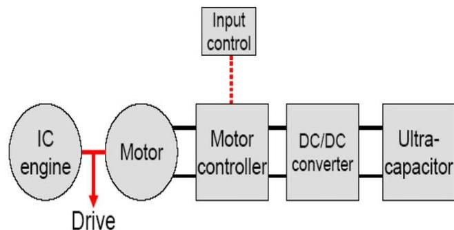
Figure.3. Regenerative Braking Systems for Use on an Electric Vehicle [4]
