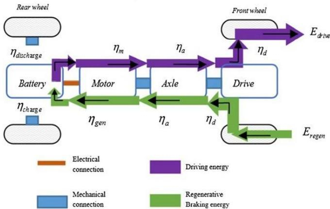
Figure.2. Energy Flow in Electric Vehicle Using Motor/Generator Unit [8]
