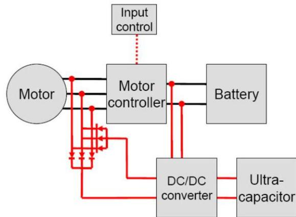
Figure.4. Regenerative Braking Systems for Use on an Electric Vehicle [4]
