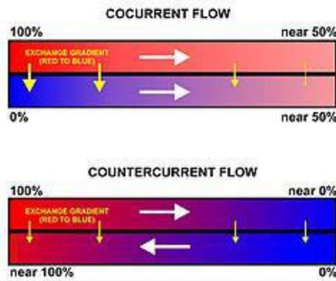
A comparison between the operations and effects of a cocurrent and a countercurrent flow exchange system is depicted by the upper and lower diagrams respectively. In both it is assumed (and indicated) that red has a higher value (e.g. of temperature) than blue and that the property being transported in the channels therefore flows from red to blue. Note that channels are contiguous if effective exchange is to occur (i.e. there can be no gap between the channels).
