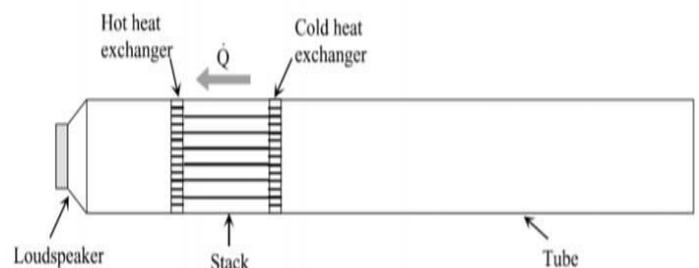
Fig. 1 Schematic representation of construction of thermoacoustic refrigerator.
