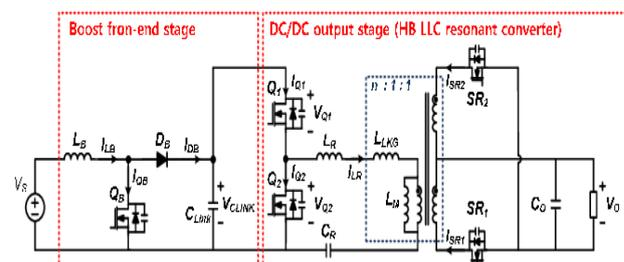
**Figure.2. Circuit diagram of two stage HB LLC resonant converter**
