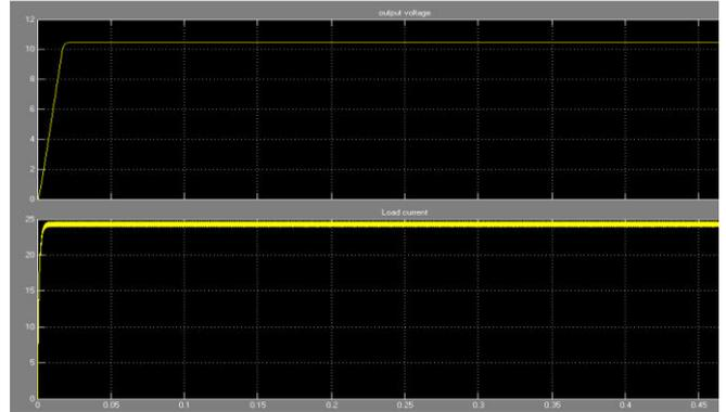
Figure.8. output voltage and load current of two stage resonant converter
