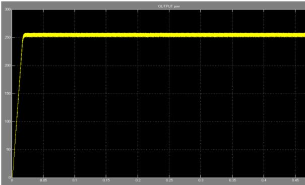
Figure. 3.6 output power of two stage resonant converter.
