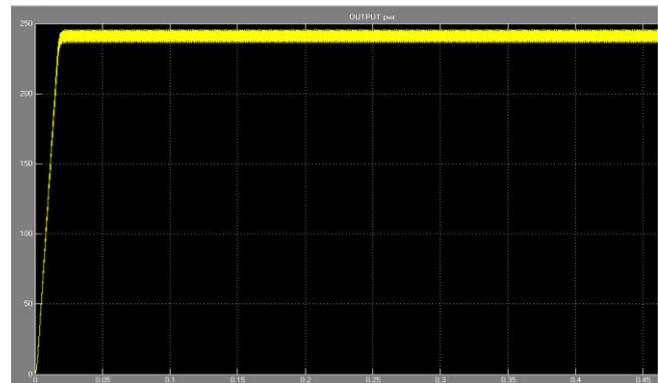
**Figure.3.2. output power of single stage LLC resonant converter**
