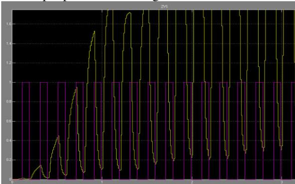
Figure.3.7 zero voltage switching in two stage resonant converter.
