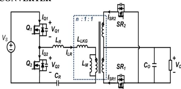
**Figure.1. Circuit diagram of single stage HB LLC resonant converter**
