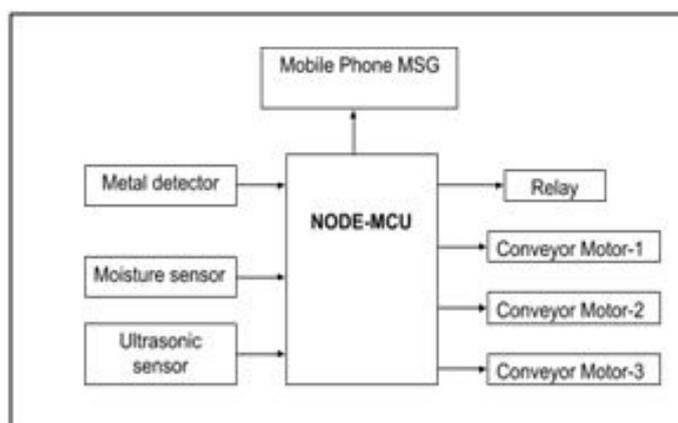
**Figure .1. Block diagram of NODEMCU**
