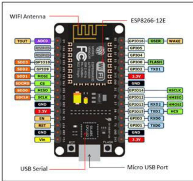
Figure .3. layout of NODEMCU
