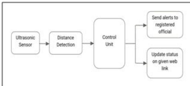
**Figure .2. Example use of ultrasonic sensor in distance measurement**
