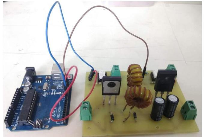
Figure. 8. 100W Prototype model of the converter
