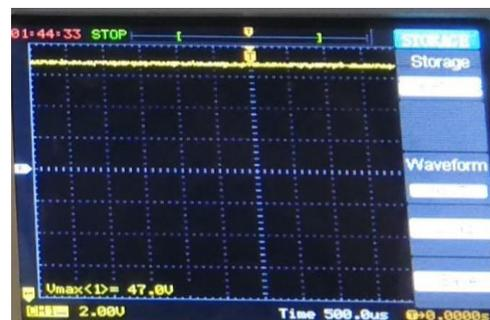
Figure.9. Output voltage of proposed converter
