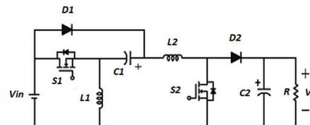
Figure.1. Proposed High gain DC-DC converter
