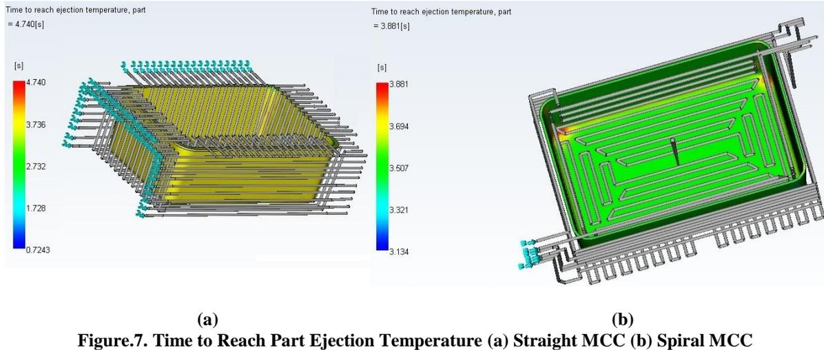
Figure.7. Time to Reach Part Ejection Temperature (a) Straight MCC (b) Spiral MCC
