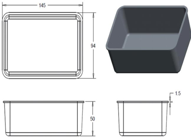
**Figure.1. Orthographic Drawing of Food Container**
