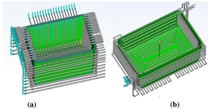
**Figure.3. Micro Cooling Channel (A) Straight Micro Cooling Channel (B) Spiral Micro Cooling Channel**
