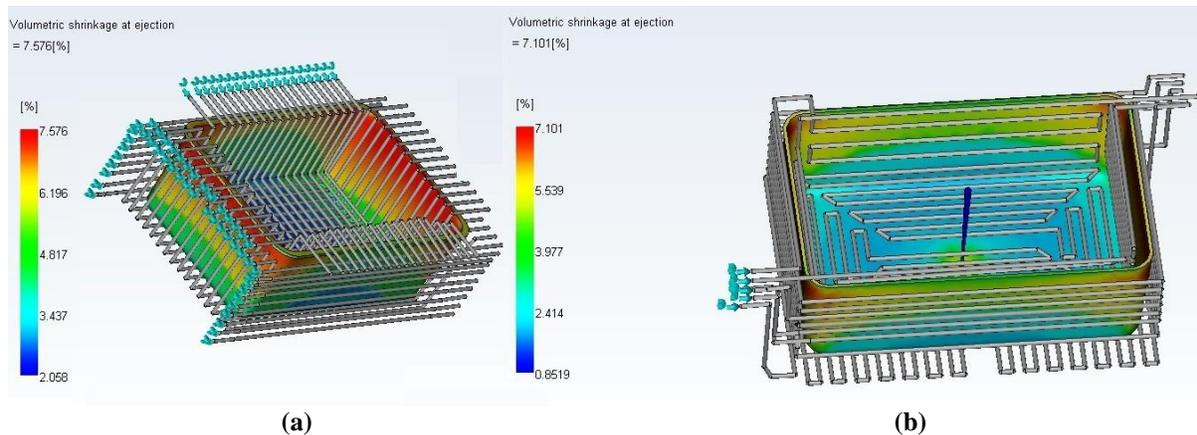
Figure.9. Volumetric Shrinkage At Ejection (a) straight micro cooling channel (b) Spiral micro cooling channel
