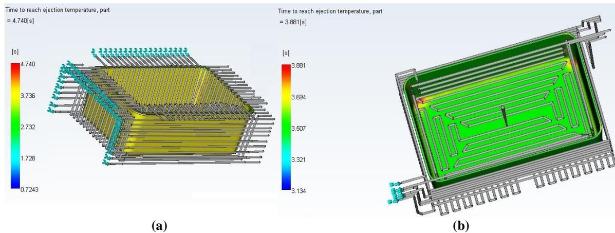
**Figure.5. Time To Reach Ejection Temperature (a) Straight MCC (b) Spiral MCC**
