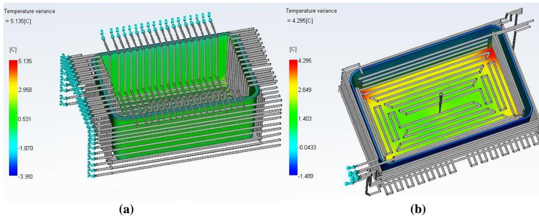
**Figure.11. Temperature Variance (a) Straight Micro Cooling Channel (b) Spiral Micro Cooling Channel**
