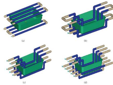
**Figure.2. (a) Conventional cooling channel design. (b) Series conformal cooling design. (c) Parallel conformal cooling channel. (d) Conformal cooling channel with additive cooling lines.**
