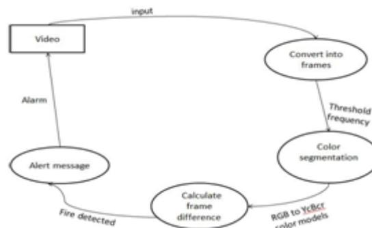
Figure.1. Proposed algorithm for fire detection
