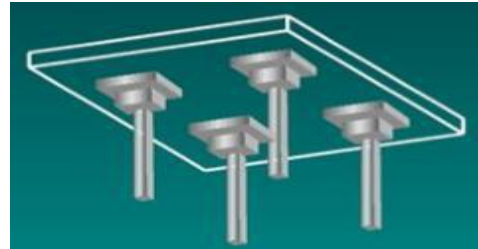
Flat Slab with Drop Panel and Column Head Figure.5. Types of Flat Slabs
