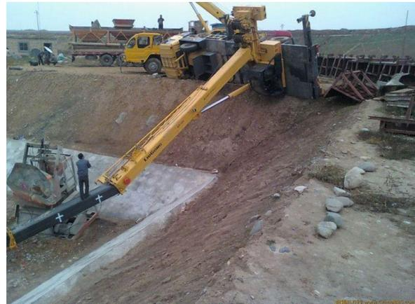
**Figure 4.3 overloading in crane accident**
