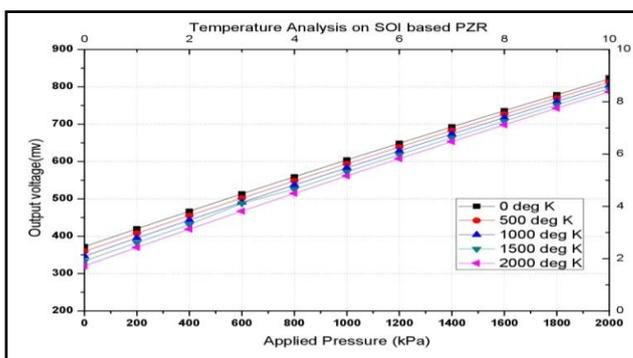
Fig 5.e: output voltage v/s applied pressure.
