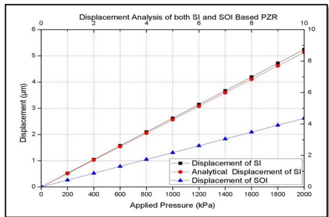
Fig 5.a: Total displacement v/s applied pressure
