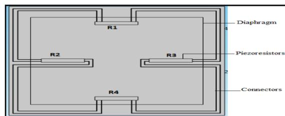
Fig 2.2 Proposed Model of SI PZR.
