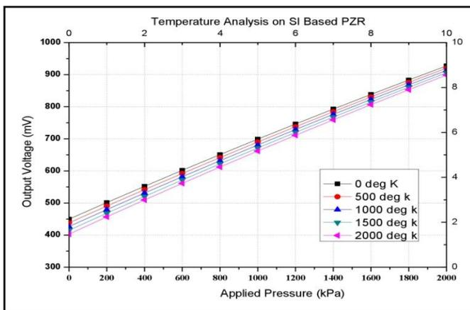
Fig 5.d: output voltage v/s applied pressure
