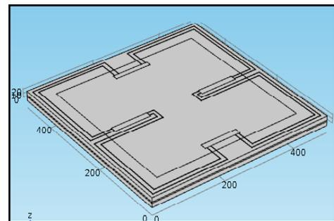
Fig 4.3 Operation of SOI based Piezoresistive pressure sensors
