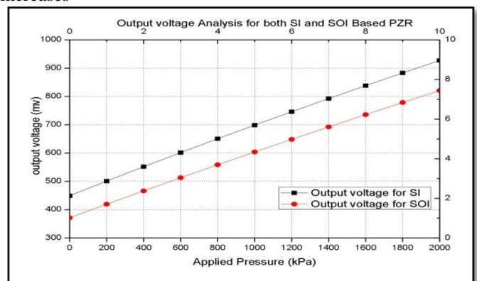
Fig 5.b: Output voltage v/s applied pressure
