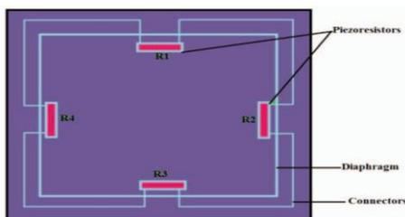
Fig 2.1: Proposed model of piezoresistive pressure sensor.
