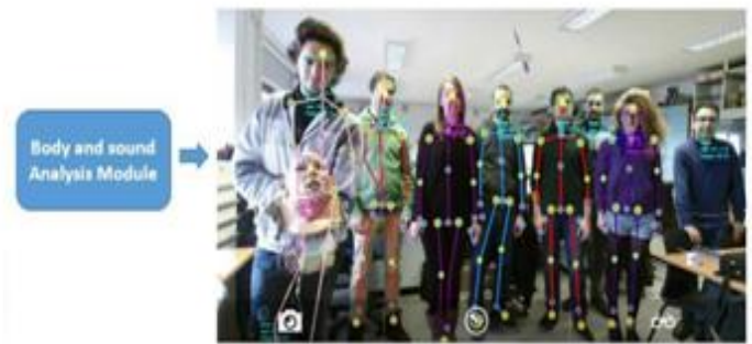
Figure.4. Multiple human tracking system: SPS detects and tracks in real time, human body and facial features. It detects also the direction of speaker comparing 3D position of human subjects and the detected sound angle (shown at the top of the figure).
