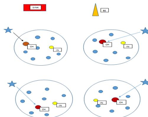
**Figure.1. Wireless Sensor Network with cluster head formation**
