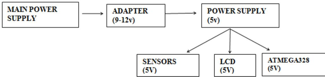
Figure.6.Flow Chart for Power Distribution
