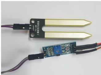
**Figure.2. Soil Moisture Sensor**
