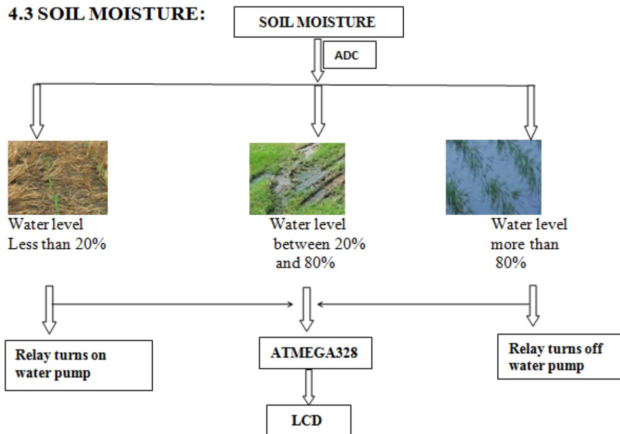
Figure.9.Flow Chart for Soil Moisture
