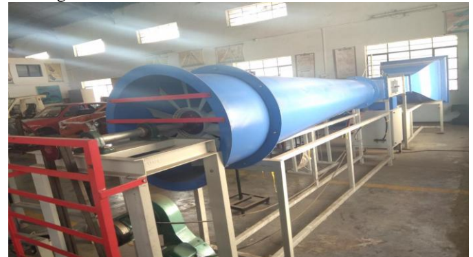
Figure 1 Open Circuit wind tunnel used for experimental investigation
