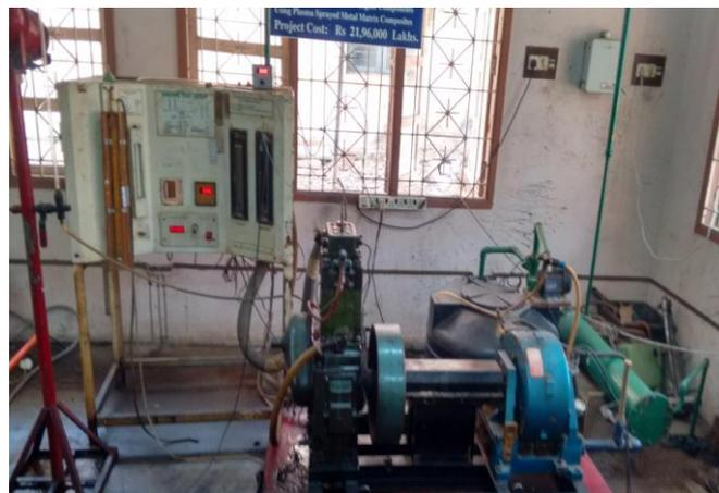
Figure 6.1 Test rig VCR research engine
