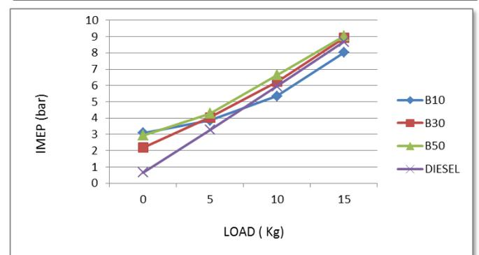
The variation of indicated mean effective pressure for various WPO diesel blend and pure diesel is shown in figure. Indicated mean effective pressure for pure diesel at 15kg load is 8.68 bar. The same for 10 %, 30 %, and 50 % WPO diesel blends are 8.02, 8.92, and 9.03 bar respectively. It is observed that indicated mean effective pressure is decreases if WPO diesel blend is increases.
