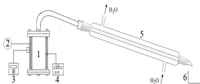
**Fig 5.1. Pyrolysis experimental set up-line diagram**
