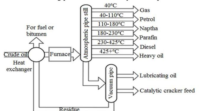
**Figure.1.1 Distillation process**
