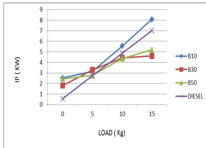
This graph shows how the indicated power is varies for 10 %, 30 %, 50% Waste plastic oil diesel blends and pure diesel. Indicated power for diesel at 15kg is 7 kW. Indicated power for 10 %, 30 %, and 50 % of Waste plastic oil diesel blend is 8.08, 4.61, and 5.18 kW respectively. It clear that indicated power is decreases if the WPO percentage in fuel is increased
