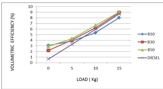
The variation of volumetric efficiency with load is shown in Figure. It can be observed from the figure that the volumetric efficiency is 75.89 % at 15kg for diesel. However when the engine is fuelled with WPO-diesel blends such as 10% WPO, 30% WPO, and 50% WPO, It gives the volumetric efficiency of 80.7%, 81.24% and 81.73%, respectively at full load. It is observed that the volumetric efficiency of the Waste plastic oil blend is closer or slightly higher to diesel except 30 % WPO diesel blend.
