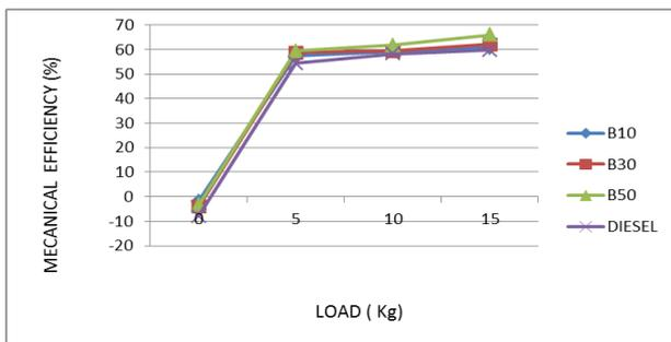
The comparisons of WPO diesel blends with pure diesel are shown in figure. Mechanical efficiency for pure diesel at 15kg load is 59.77 %. The same for 10 %, 30 %, and 50 % WPO diesel blends are 60.79 %, 62.1%, and 65.99% respectively. It is observed that for all WPO diesel blends mechanical efficiency is higher when compared to pure diesel. It is also observed that the mechanical efficiency is increased from 60.79 to 62.1 % for 30 % WPO diesel blend from 10 % WPO
