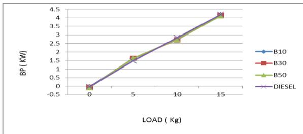
This shows how the brake power is varies for 10 %, 30 %, 50% Waste plastic oil diesel blends and pure diesel. Brake power for diesel at 15kg is 4.19 kW. Indicated power for 10 %, 30 %, and 50 % of Waste plastic oil diesel blend is 4.17, 4.11, and 4.23 kW respectively. It is observed that brake power for different blends is higher as compared to pure diesel.
