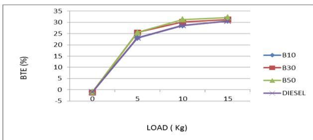
The variation of brake thermal efficiency with load is shown in Figure. It can be observed from the figure that the thermal efficiency is 30.56% at 15kg load for diesel. However when the engine is fuelled with WPO-diesel blends such as 10% WPO, 30% WPO, 50% WPO, it gives the thermal efficiency of 30.66%, 31.25%, 32.16 % respectively at 15kg load. It is also observed that brake thermal efficiency is higher for 10%, 30 % and 50% WPO when compared to pure diesel.
