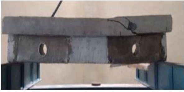
Figure.15. Failure Pattern of strengthened Beam at ultimate load
