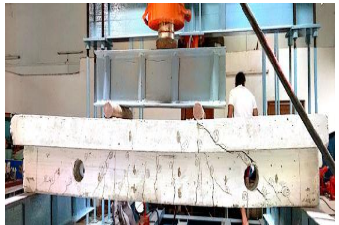
Figure.14. Failure Pattern of Unstrengthened Beam at ultimate load
