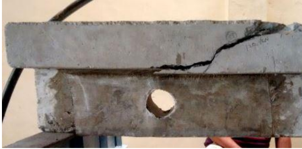
Figure.16. De-lamination of GFRP of Strengthened Beam
