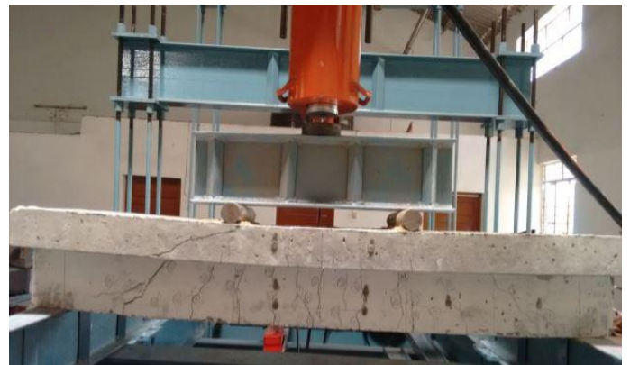
Figure.13. Failure Pattern of Control Beam at ultimate load
