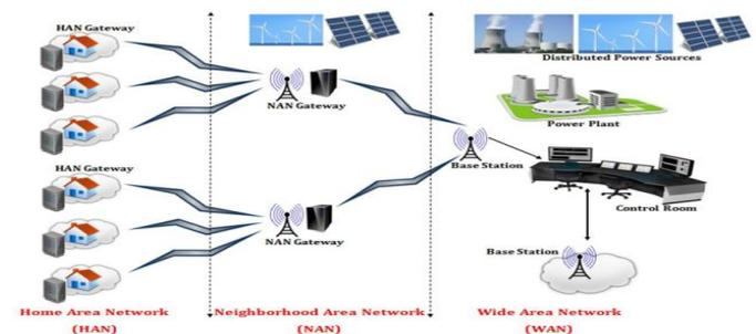
**Figure.1. Classification of Smart Grid Communication Networks**
