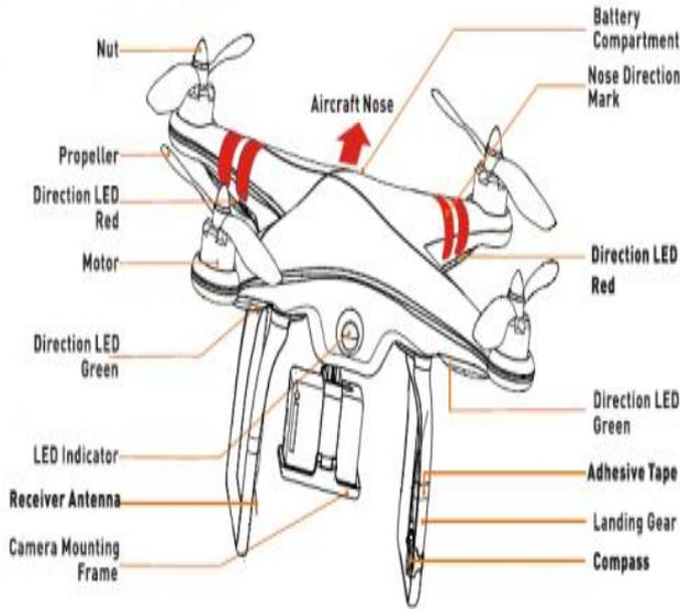
Figure.2. Components of quad copter
