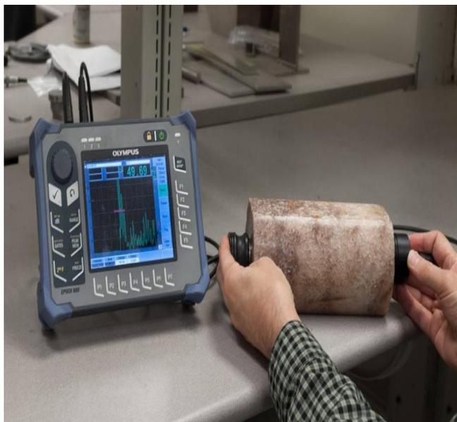
Figure.4. Ultra pulse velocity instrument
