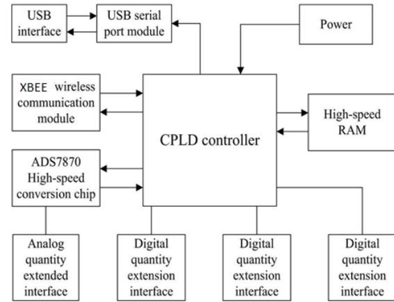
Figure 4. CPLD hardware block diagram
