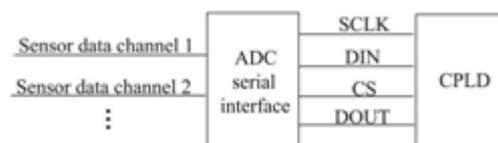
**Figure.2. Independent sensor interface function schematic.**
