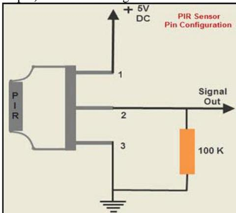
Figure.7. Pin configuration of PIR sensor
