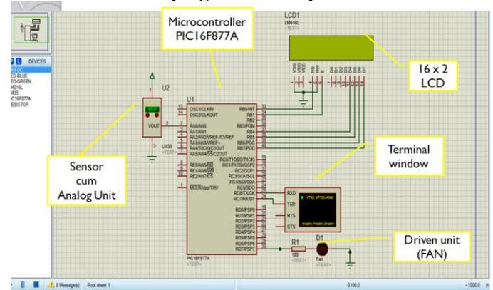
This is the simulation program for temperature sensor using PROTUES software. The sensor cum analog unit used to change the input/temperature. The microcontroller program written using MPLAB IDE. The WINPIC is a booting tool for microcontroller. We can see the real time dates in 16x2 LCD. We can see what dates are passed to the CPLD in terminal window. In WSN 1 our driven unit is fan.
