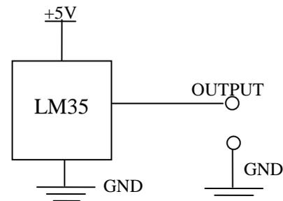
Figure 5. Circuit diagram for the LM35 temperature sensor functional module
