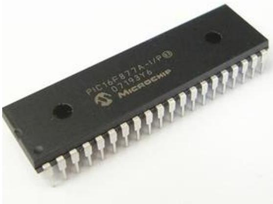
Figure.8 .PIC 16f77a microcontroller
