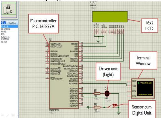
This is the simulation program for PIR sensor using PROTUES software. Here the input unit is sensor cum digital unit. When the switch is ON the driven unit Light is ON. When the switch is in OFF condition the Light is OFF.
