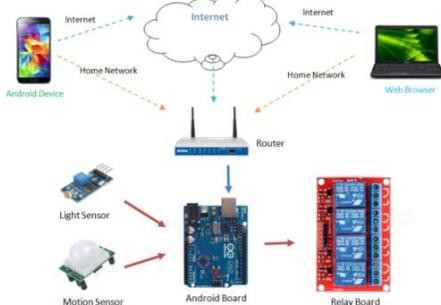
Figure.1. Overall system layout
