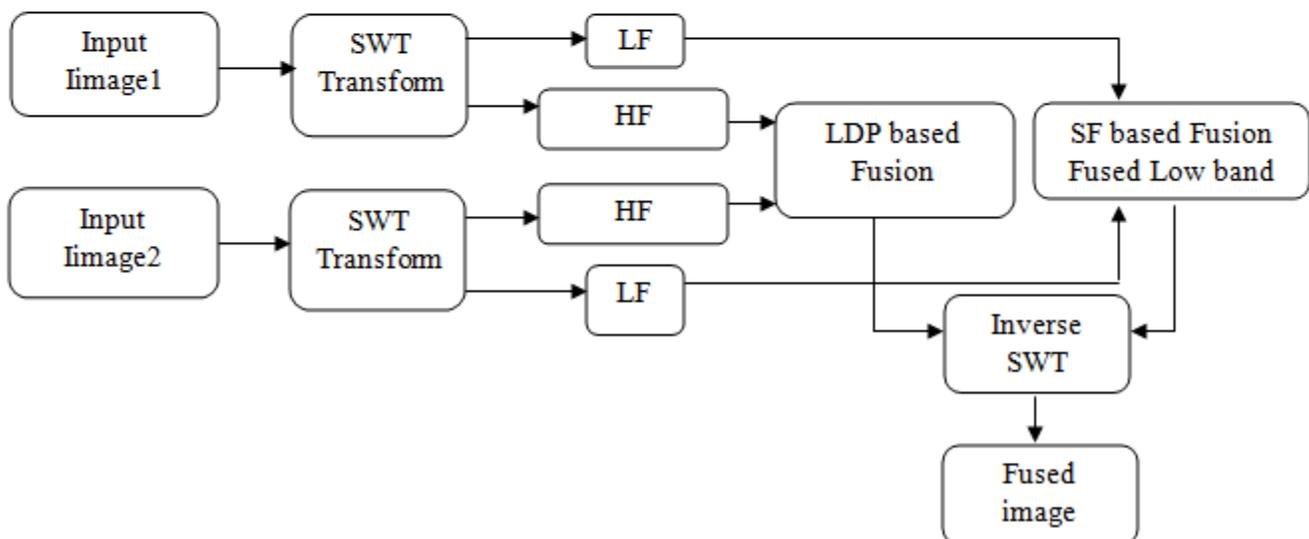
Figure.1. Proposed Method Block Diagram Using SWT Method:-
