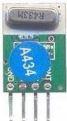
Figure.1. RF Transmitter
