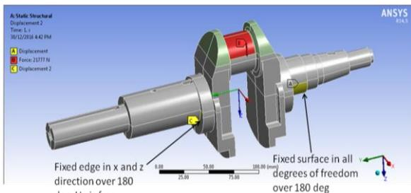
**Figure.3. Loading and boundary conditions**
