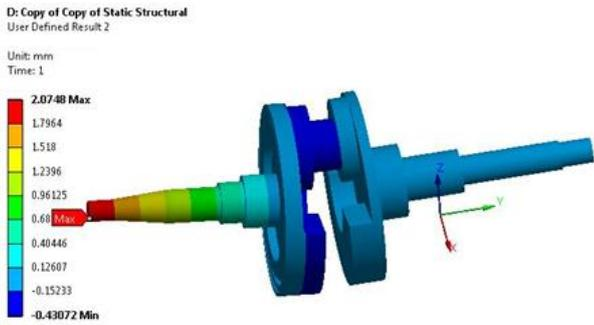
**Figure.8. Displacement Contour plot**
