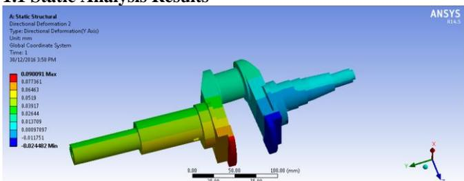
**Figure.4. Displacement Contour plot**
