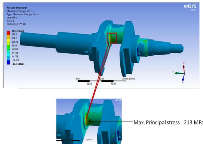
**Figure.5. Contour Plot for Max Principal Stress**
