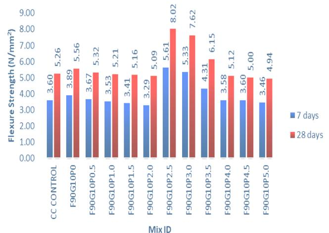
Figure.6. comparison of flexural strength test
