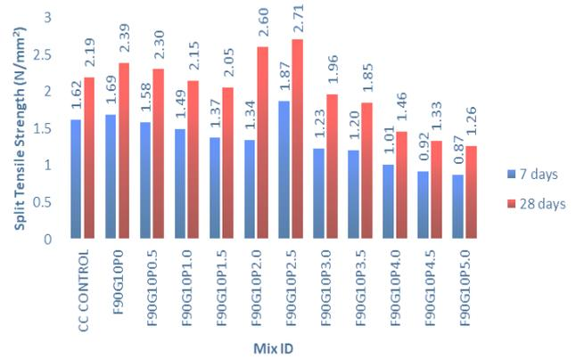
Figure.5. Comparison of Split Tensile Strength
