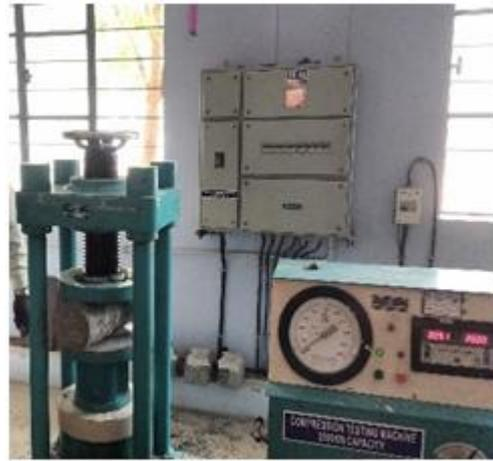
Figure.2. testing of gpc cylinders
