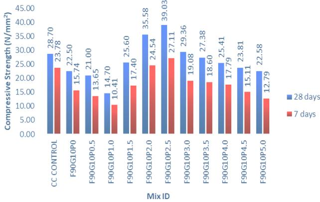
Figure.4. comparison of compressive strengths
