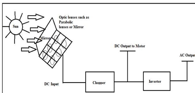
**Figure.2. Block diagram of developed system**
