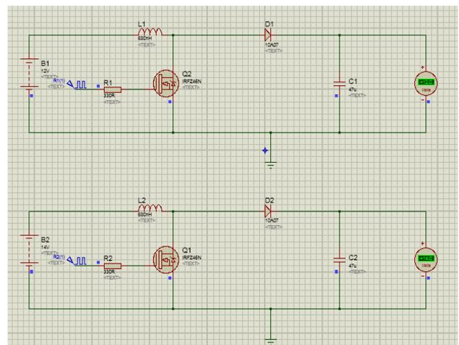
Figure.7. Simulation output of DC Boost converter
