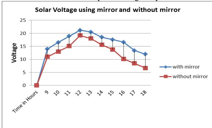
Figure.10. Solar panel voltage with and without mirror
