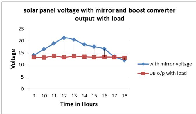
Figure.9. Graph of solar panel voltage with mirror and boost converter output with load
