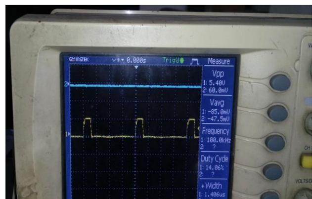
Figure.8. DC boost circuit output
