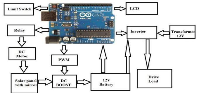
**Figure. 3. Circuit diagram of developed system**
