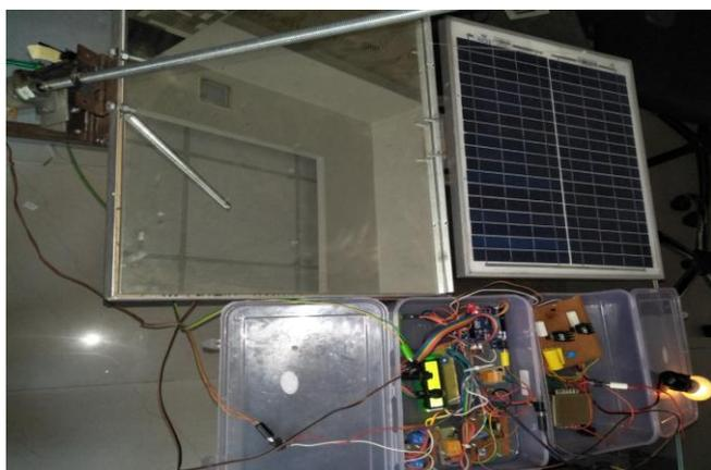
Figure.5. Our Experiment solar panel with auto rotate mirror
