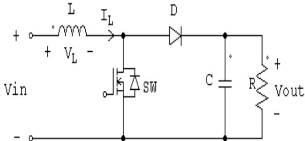
Figure.4. Schematic of Boost Converter
