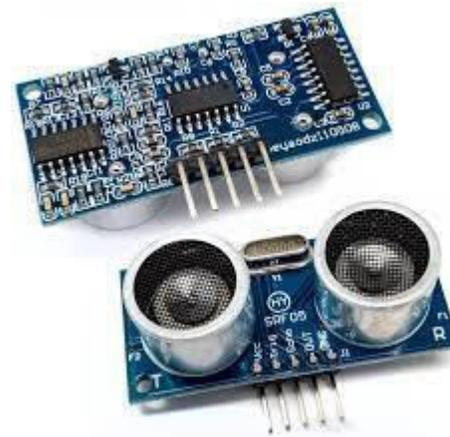
**Figure.2. Ultrasonic Sensor**
