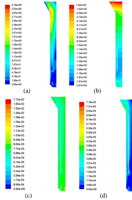
Figure.7. (a) air velocity contour (b) pressure contour (c) glucose mass fraction (d) PHB mass fraction, of the case study.
