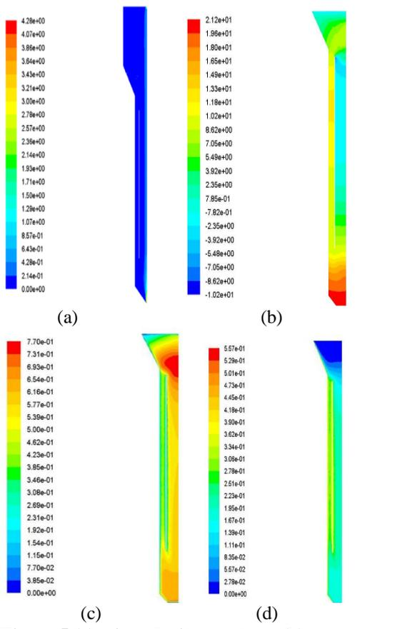
Figure.5.(a) air velocity contour (b) pressure contour (c) glucose mass fraction (d) PHB mass fraction, of validated model
