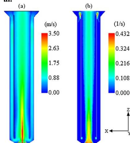
**Figure.4. Profile of (a) liquid velocity in the bioreactor (b) volumetric oxygen transfer coefficient calculated by Eqn 42 at aeration rate of 30 L/min data by Poorya Mavaddat et al.**
