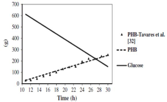
**Figure.2. Variation of the modeled polyhydroxybutyrate and glucose and experimental data by Tavares et al.**
