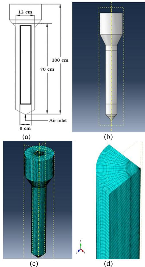
**Figure.1. (a) Shows schematic diagram of airlift bioreactor (b) pre-processor model (c) hexahedral mapped model (d) symmetric view of hexahedral model**
