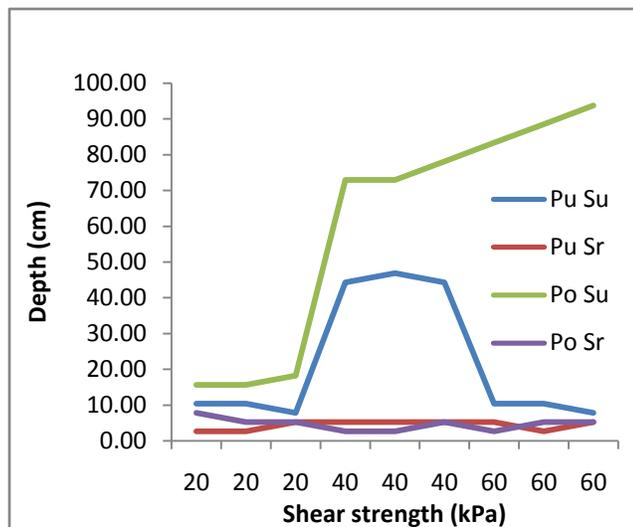
Fig. 3. Variation in undisturbed shear strength (Su) and remoulded shear strength (Sr) over depth at the test sites
