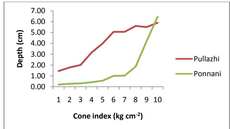
Fig. 2 Variation in cone index with depth
