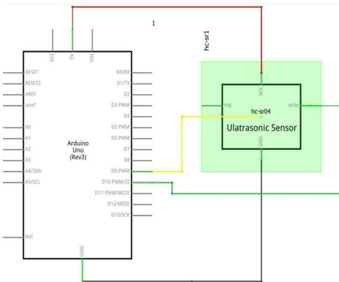
Figure.2. Interfacing of Arduino with Ultrasonic Sensor
