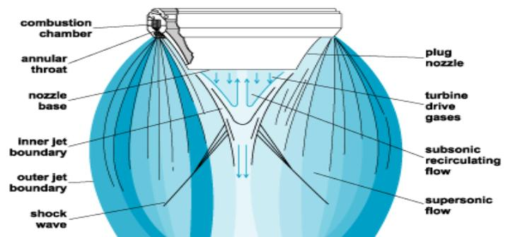
**Figure. 1. Flows around Spike Nozzle**
