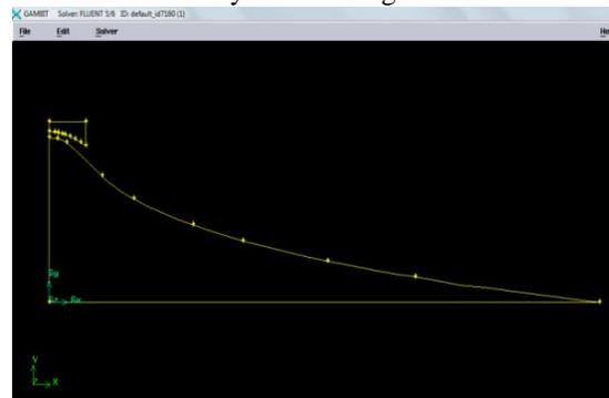
**Figure.7. Gambit design of spike nozzle**
