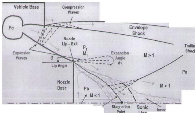
**Figure.3. Exhaust Flow along a Truncated Spike Nozzle**
