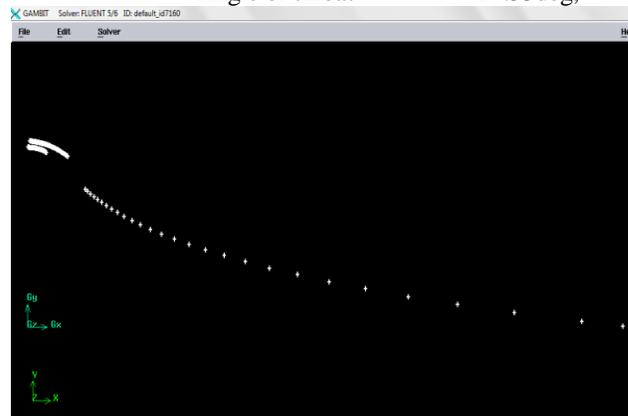
**Figure.6. Gambit design of spike nozzle**
