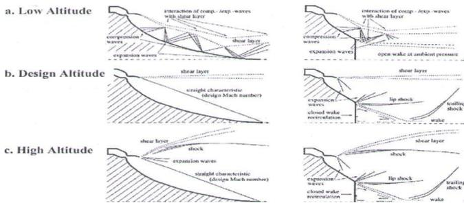
**Figure.2. Exhaust Flow from a Full and Truncated Spike**
