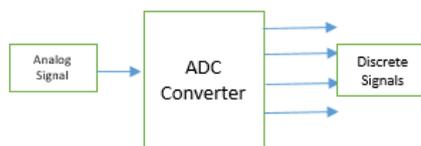
Fig 3.1.1: Block Diagram of ADC
