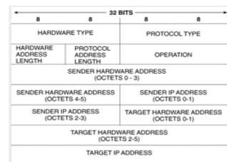
Fig 1.2 ARP Packet Format [2]
