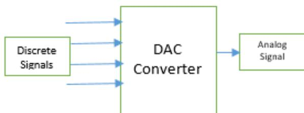
Fig 3.2.1 Block diagram DAC
