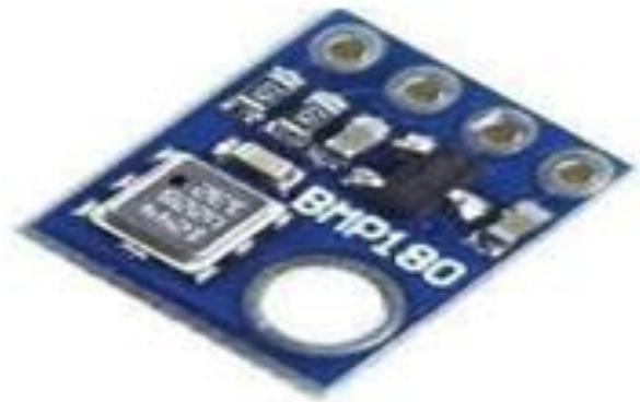
**Figure.7. pressure sensor**
