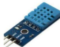
**Figure.5. temperature and humidity sensor**
