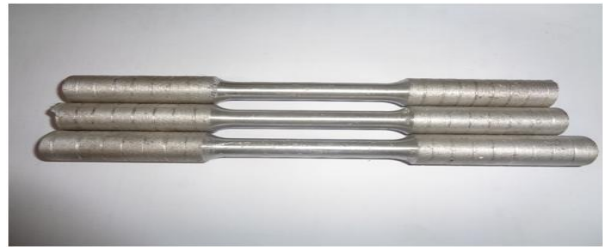
Figure.2.1 After Machining in standard dimensions
