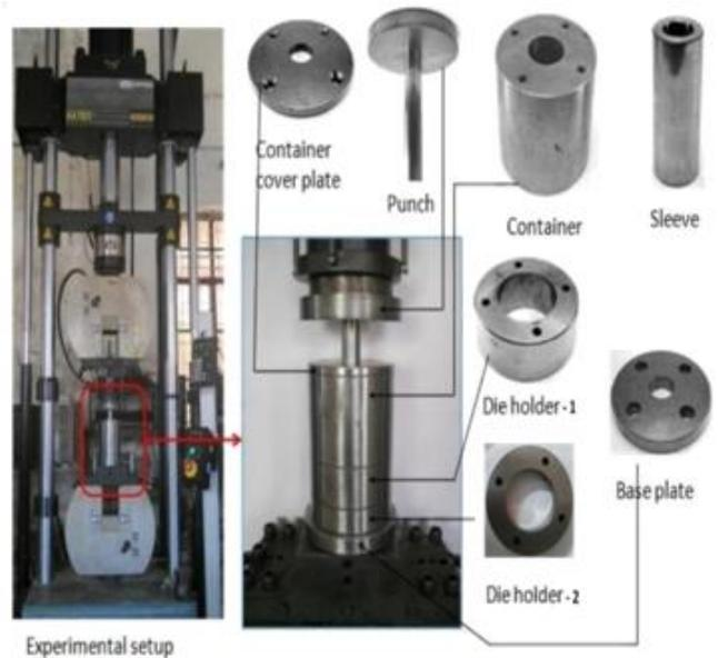
Figure.2. Photographic view of experimental setup with main components
