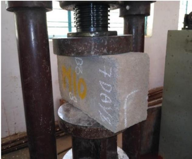
Three specimens (blocks) from each type of mix proportions, cured for 7 days and 28 days, the compression test is carried out on specimen cubical, cylindrical in shape and prism shape. The block specimen is of the size 200X150X400mm
