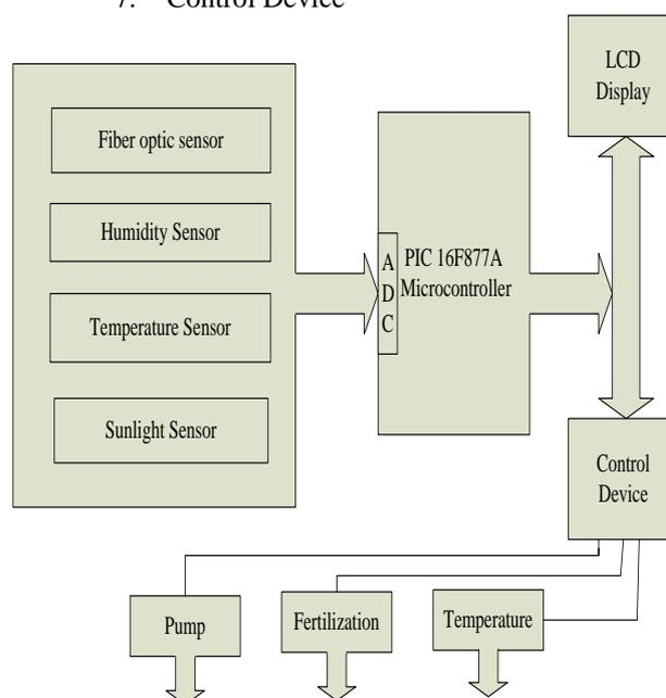
Figure.1. Proposed system diagram
